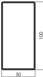
100×50 Rectangle Beam Thickness:1.8/2.0mm
